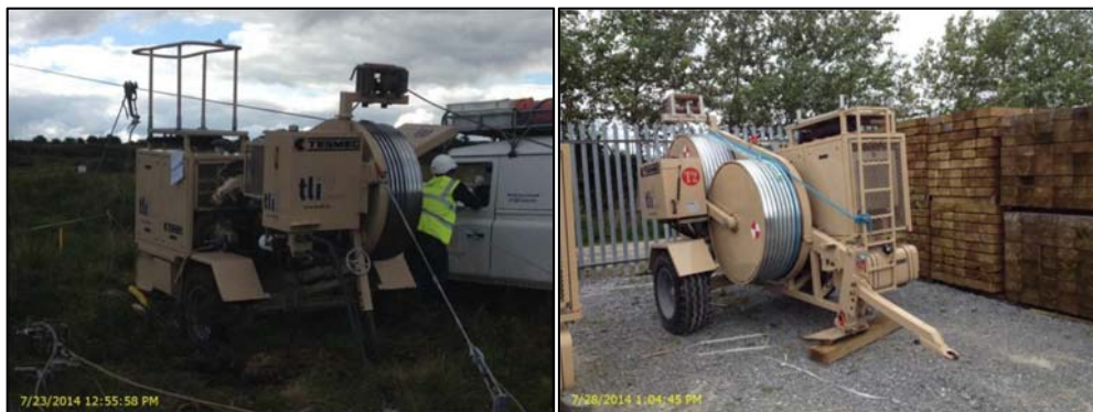
Plate 4.12 Puller – Tensioner Machine
